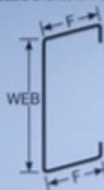
Eave Strut double broke, low side
